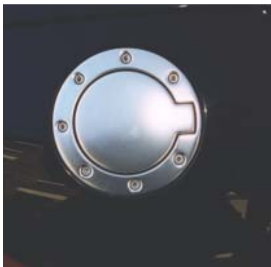
Fig. 10 Joining as a means of expression. The precision-machined stainless steel fuel cap on the left, attached by eight Allen screws (it carries no significant loads) projects a sense of the precise engineering of the entire vehicle. The watch on the right uses the same motif to suggest that it is built to resist the harshest treatment.
